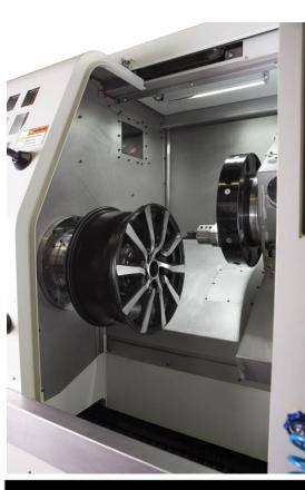
The Efamatic BT-22 CNC Lathe has been designed and engineered from the ground-up for the specific task of Bright and Diamond Turning.
