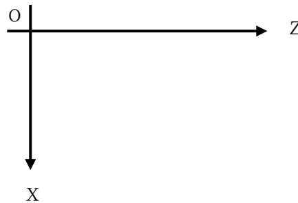
Fig. 1-1 X—Z plane rectangular coordinate system 1 (front tool post coordinate system)
