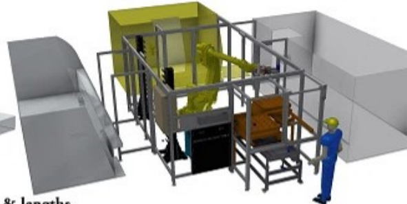
COMPLETE CELLS: Turnkey setups including fencing, loaders & grippers
