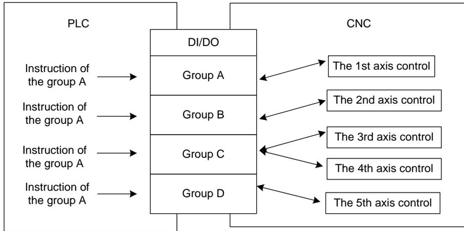
Fig.9.1 PLC axis control diagram
