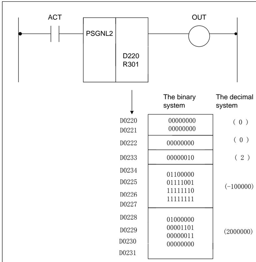
For the above ladder diagram and control data, if ACT=1, when  $-100.000 \leq 2^{\text{nd}}$  axis position in machine coordinate  $\leq 200\text{mm}$ , OUT=1.
