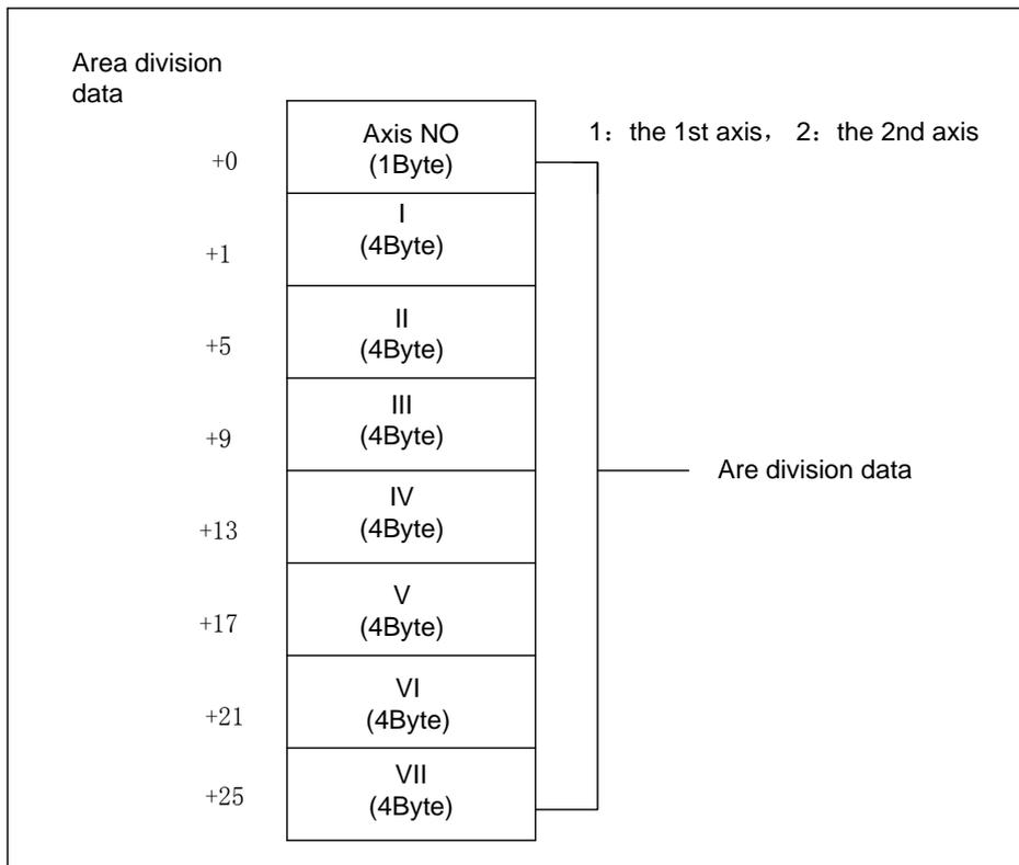
Axis No sets axis number (a binary one-byte data)
