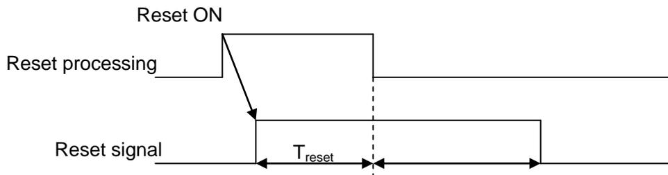
When the CNC is reset during automatic operation, automatic operation is stopped and is decelerated to stop. When the CNC is reset during the execution of the MF, SF or TF signal is set to 0 within 16ms.
