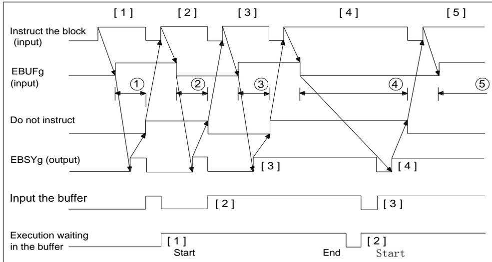
Fig. 9.3 PLC axis control command sequence diagram
