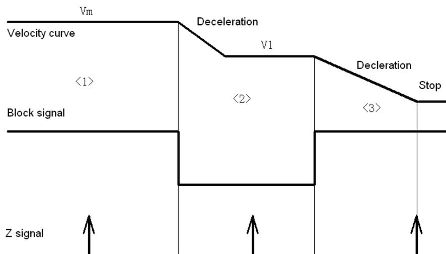
Fig. 4-1 The process of manual reference return
