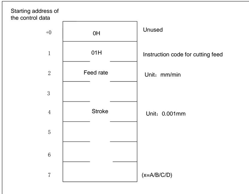
**Note: relevant CNC parameter for axis move must be set.**
