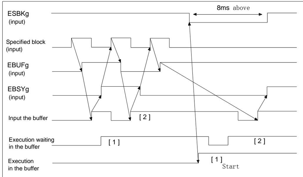
Fig. 9.4 Relevant signal sequence diagram to P block stop
