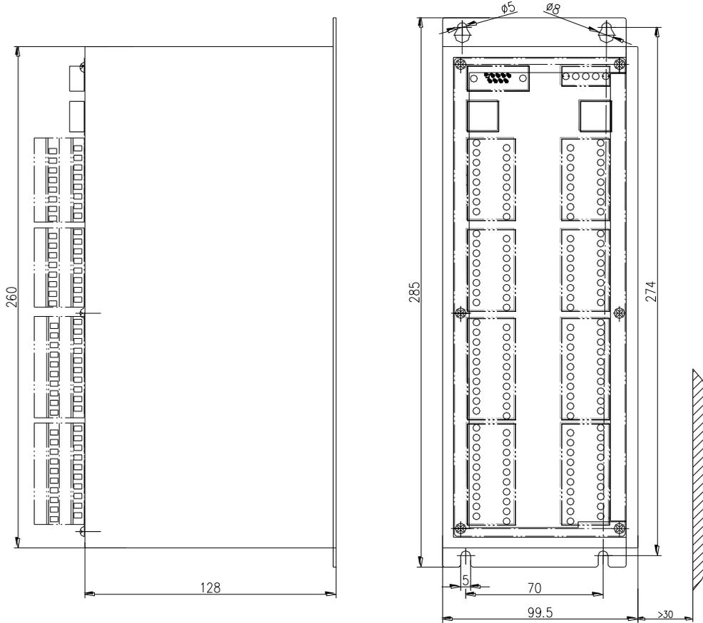
**4.8 External position detection unit GSK25i-PDU installation dimension**
